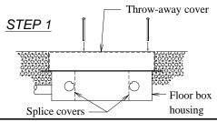
Set floor box housing in position for concrete pour and remove splice cover. Run feed wires and connect conduit. Install throw-away cover. Level with finish concrete surface, and pour concrete. Sides of throw-away cover should be treated for easy removal after conrete has hardened. Note: Axis of rotation of cast brass assembly will be parallel to the 11" dimension of floor box housing.
