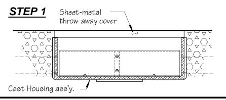
Set housing in position for concrete pour with conduit connected & with THROW-AWAY COVER ATTACHED. Throw-away cover must be flush (level) with finished concrete surface. Sides of cover should be suitably treated to facilitate removal after concrete is set.
