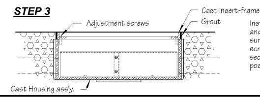
Install cast insert-frame and level to finished concrete surface by means of adjustment screws. Grout all around, securing insert-frame in final position to receive cover.
