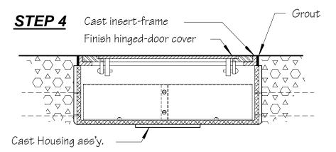
Full branch-circuit wiring into housing, connect to devices mounted on interior panel, & secure finish hinged-door cover in place with flat head screws provided.
