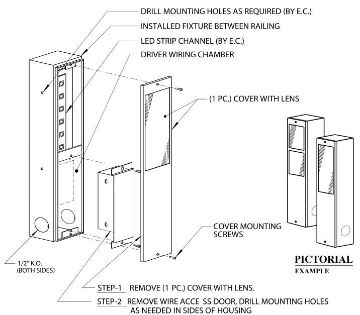
STEP-3 CONNECT CONDUIT TOK.O. ON ONE OR BOTH SIDES TO INSTALL & WIRE. (BY E.C.)
